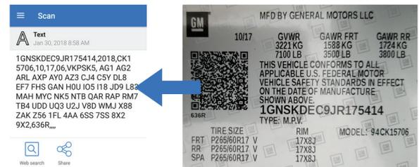
A Service Parts Identification (SPID) Label provides Vehicle Identification Number (VIN)-specific Option Code content list, Engineering Model Number (Nameplate, body style), Exterior paint system, Exterior paint color code and Interior trim level and color.
