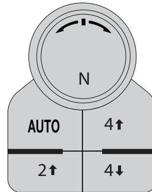
Active, 2-speed electronic Autotrac with rotary controls, includes neutral position for dingy towing. Use the transfer case knob next to the steering wheel to shift into and out of four-wheel drive.
