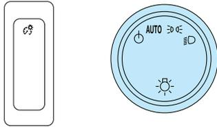
The headlamp control on the driver's side of the instrument panel operates the exterior lamps. If your Silverado does not have option 9G8, DELETE DAYTIME RUNNING LAMPS and AUTOMATIC HEADLAMPS, the Daytime Running Lamps and Automatic Headlamps can be turned OFF for one ignition cycle by rotating the headlamp control knob momentarily counter-clockwise. See your Silverado Owner's Manual.
